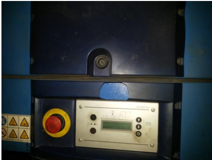
Localized air compressor helps reduce overall system pressure
